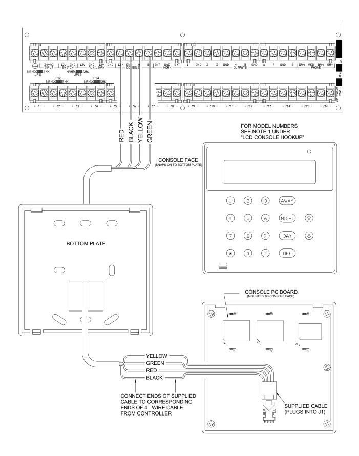
FIGURE 6 - CONSOLE CONNECTIONS
