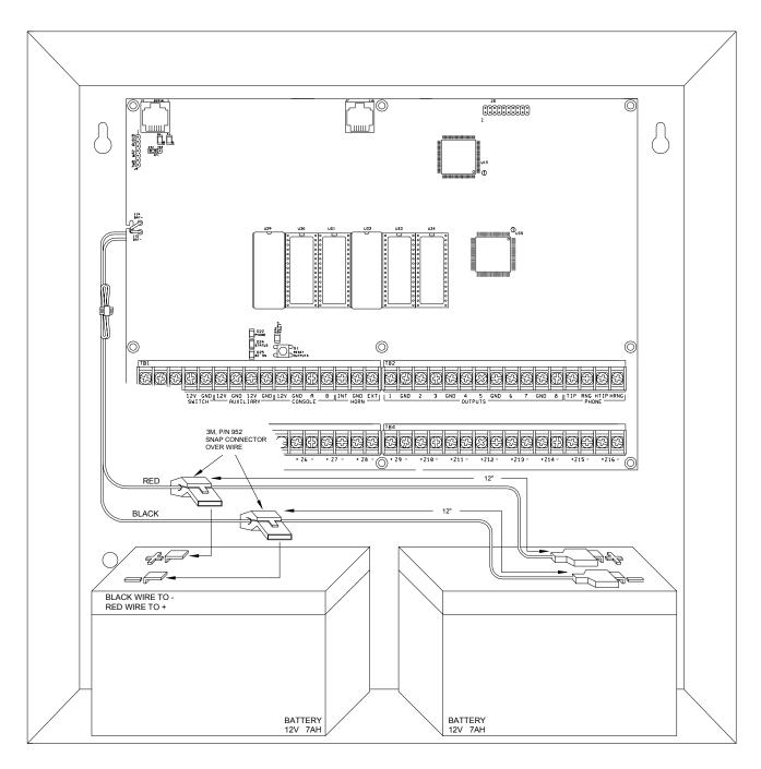
FIGURE 15 - 24-HOUR STANDBY CONNECTIONS
