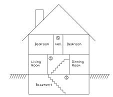
A smoke detector should be located on each story.
