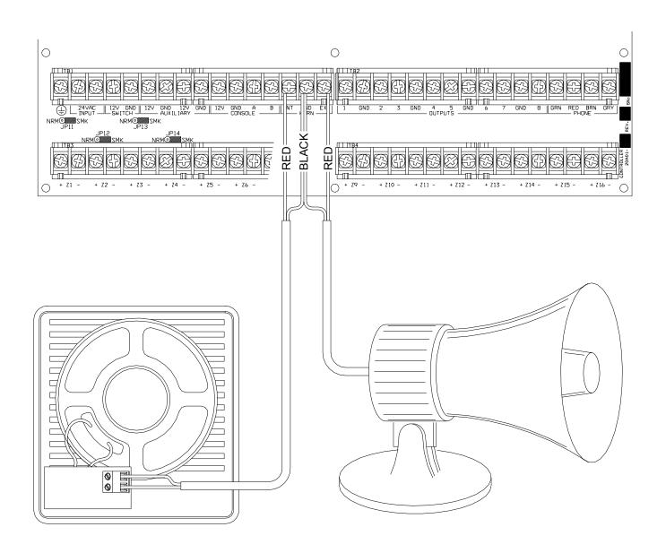
**FIGURE 7 - SOUNDER CONNECTIONS**
