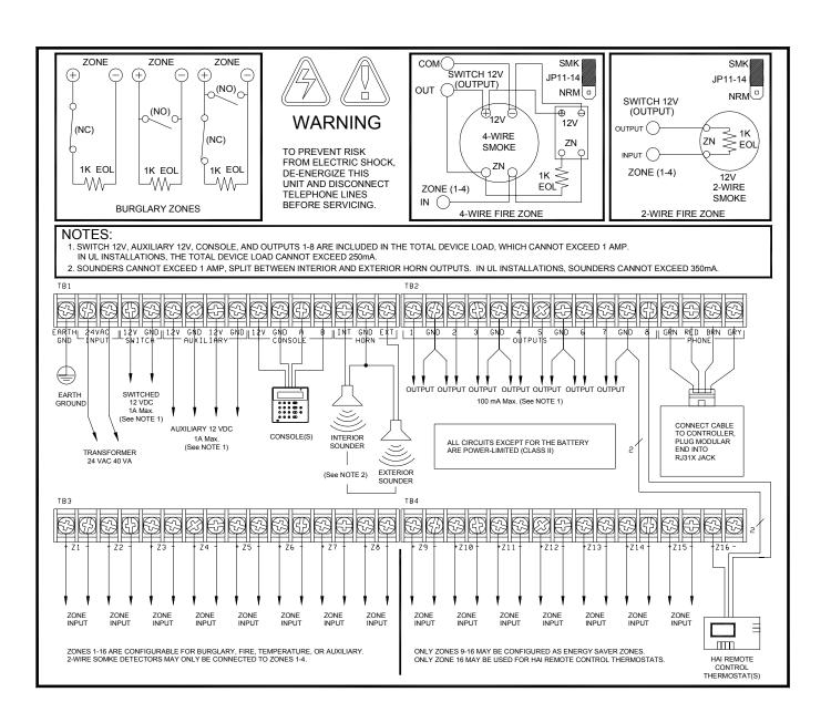
FIGURE 2 - OVERALL CONNECTIONS DIAGRAM
