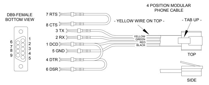
FIGURE 13 - RS-232 CONNECTIONS
