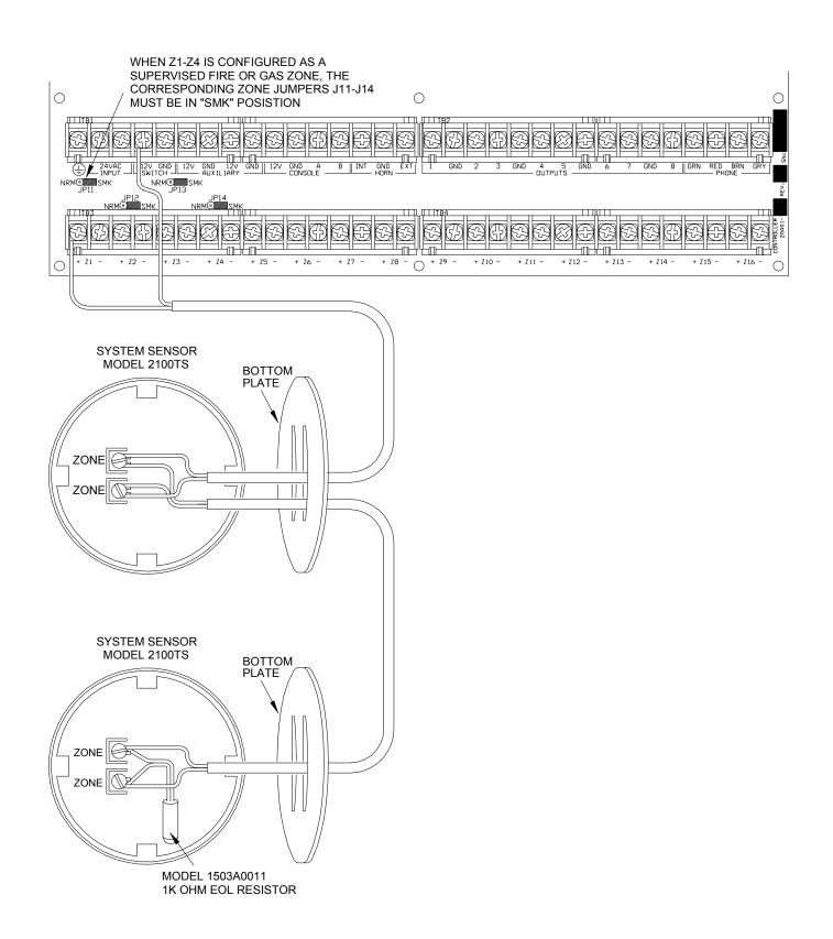
FIGURE 3 - TWO-WIRE FIRE ZONE CONNECTIONS
