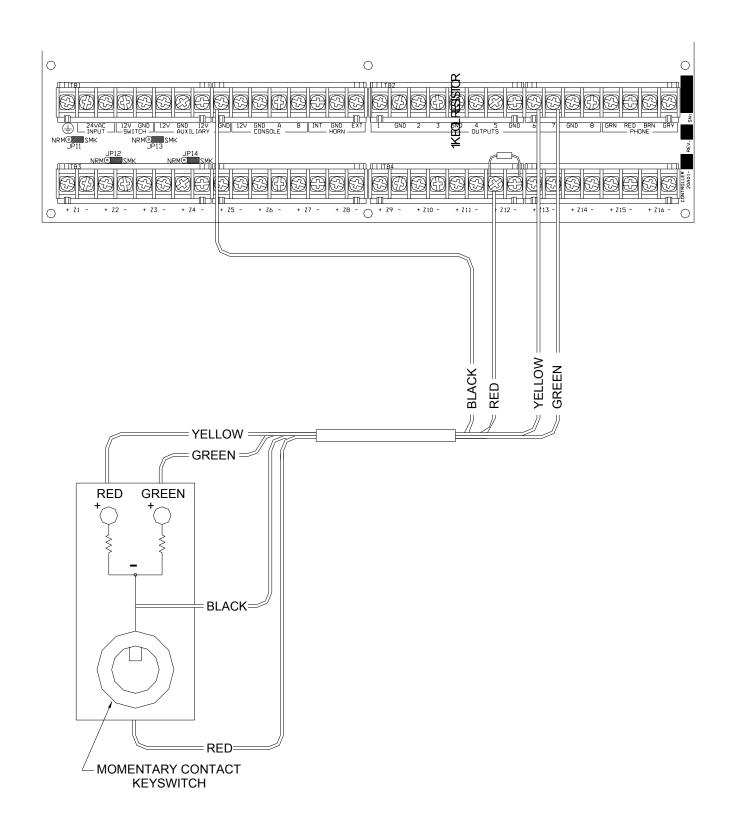
FIGURE 9 - REMOTE KEYSWITCH CONNECTIONS
