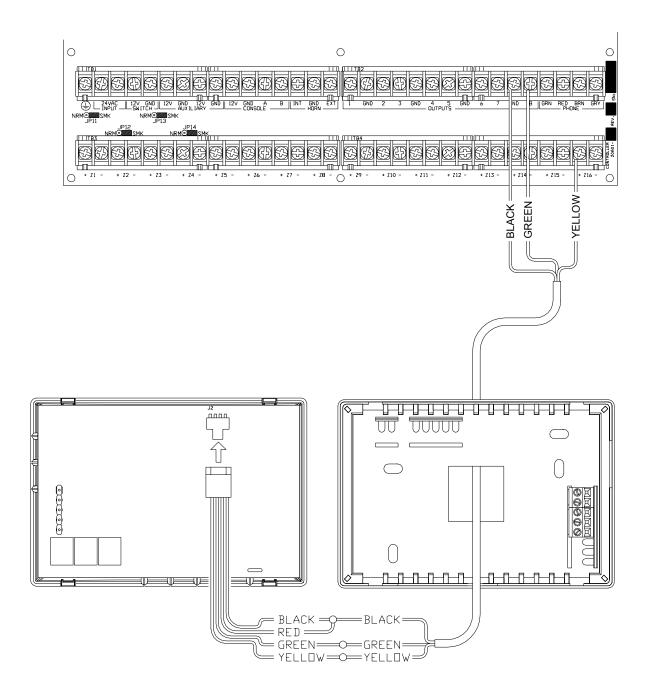
FIGURE 10 - HAI THERMOSTAT CONNECTIONS
