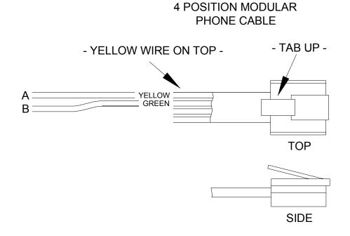
FIGURE 14 - RS-485 CONNECTIONS
