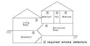
Split level arrangment. Smoke detectors are required where shown. Smoke detectors are optional if door is not provided between living and recreation rooms.
